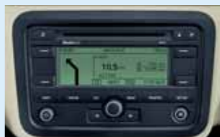
Navigation system with dynamic TMC module: enabling reception of traffic information, RDS-equipped AM/FM receiver, CD and MP3 player, connection to a CD changer, input jack for the mobile phone hands-free set.
