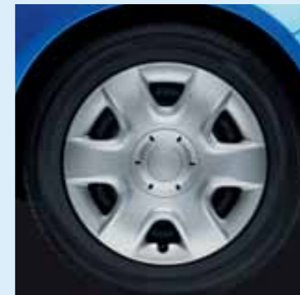
6.0J x 15" steel wheels for 195/55 R15 tyres with Hermes hub covers.
